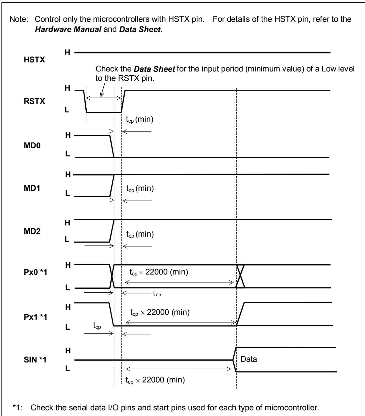
Minimum values of setup and hold times of each signal on rising edge of RSTX
