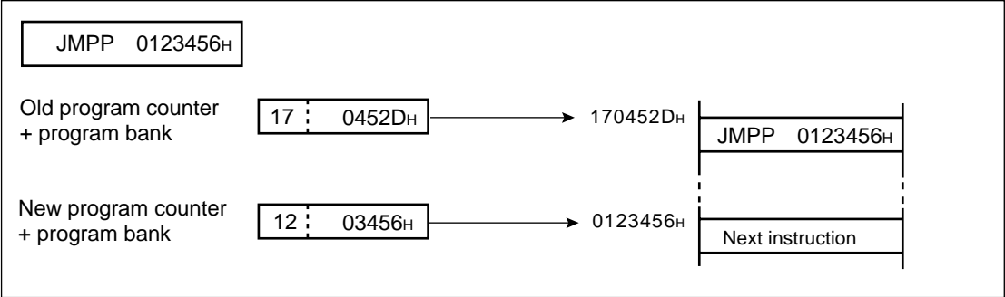
Figure 2.4-2 Example of Direct Specification of a 24-bit Physical Address in Linear Addressing
